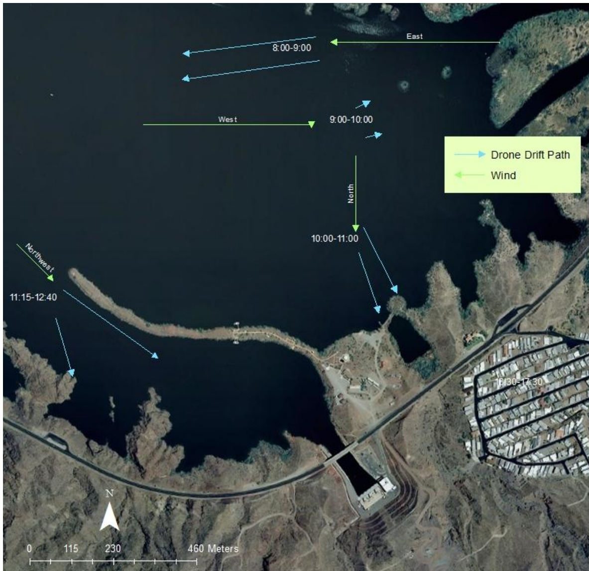
Figure 38. Morning drone drift paths and predominant wind direction observed in Bill Williams NWR on October 4, 2012. The length of the arrow tail is the scaled distance the drones traveled.
