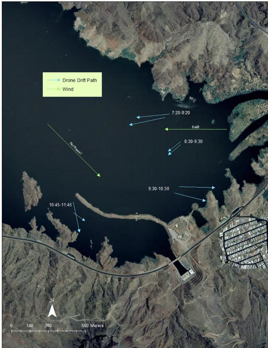
Figure 32. Morning drone drift paths and predominant wind direction observed in Bill Williams NWR on October 2, 2012. The length of the arrow tail is the scaled distance the drones traveled.
