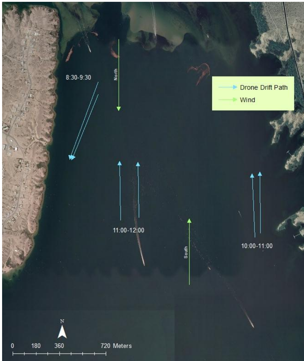
Figure 29. Morning drone drift paths and predominant wind direction observed near the Colorado River inflow in Lake Havasu on October 1, 2012. The length of the arrow tail is the scaled distance the drones traveled.
