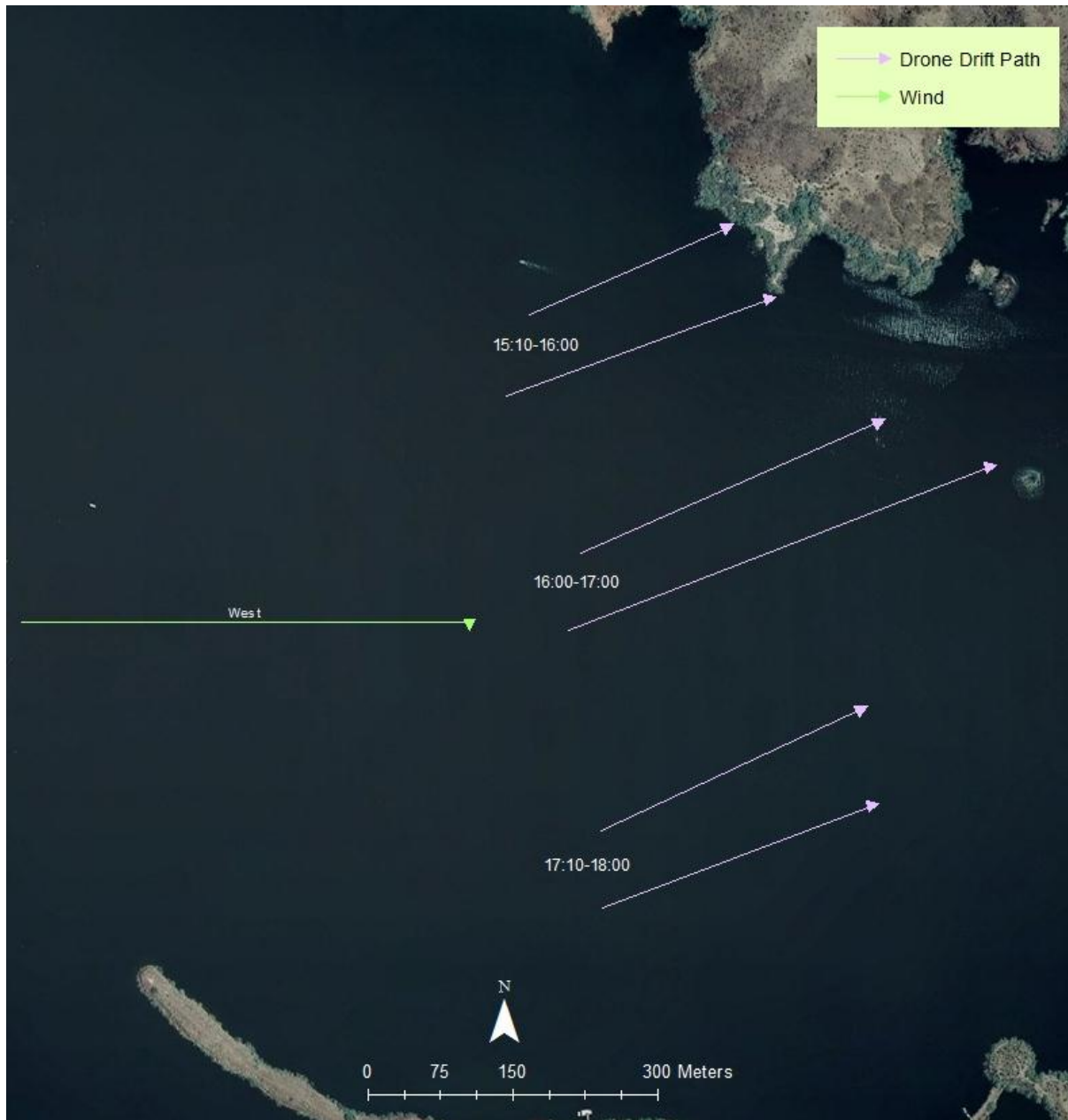
Figure 40. Afternoon drone drift paths and predominant wind direction Bill Williams NWR on October 4, 2012. The length of the arrow tail is the scaled distance the drones traveled.
