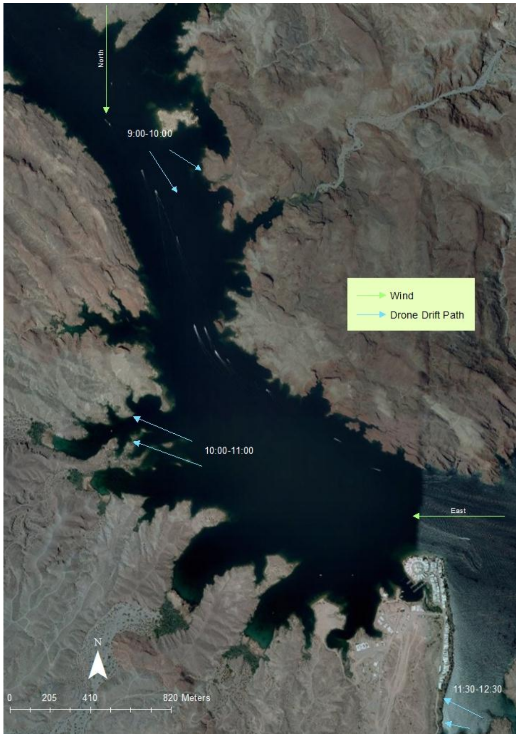
Figure 36. Morning drone drift paths and predominant wind direction observed in river-like area of Lake Havasu that flows into Bill Williams NWR on October 3, 2012. The length of the arrow tail is the scaled distance the drones traveled.
