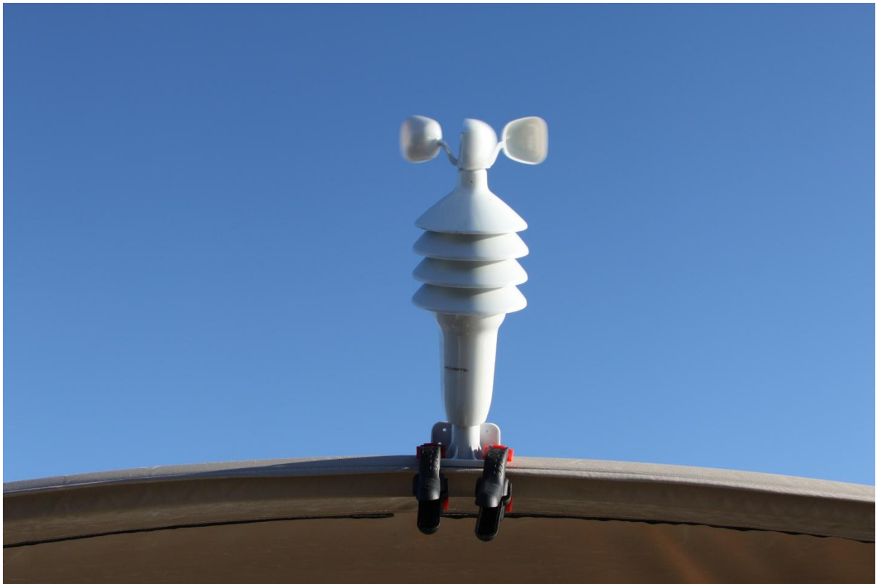
Figure 6. On board weather station that recorded average wind speed. Photo by John D. Madsen.
