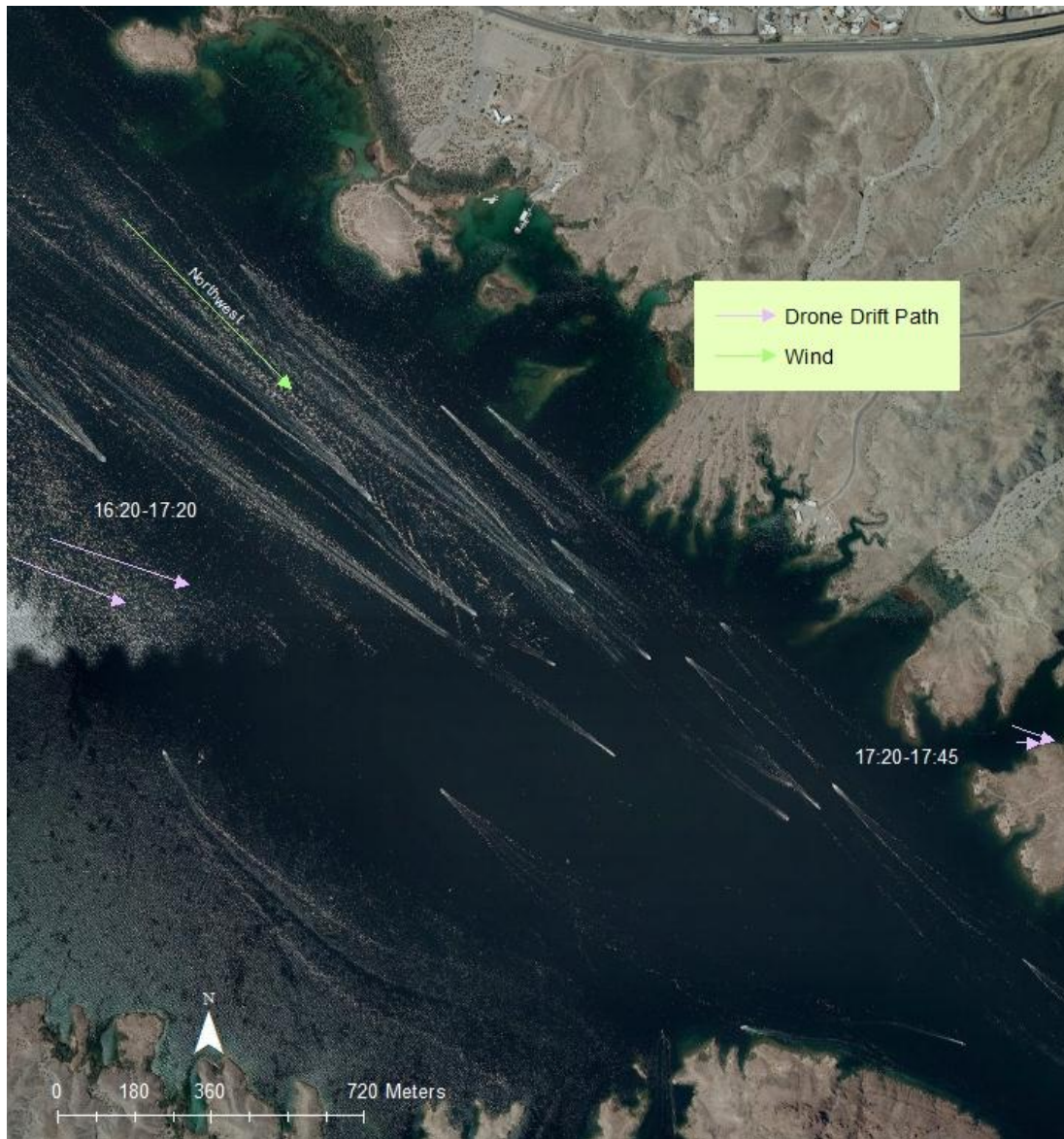
Figure 31. Afternoon drone drift paths and predominant wind direction observed near the entrance of the river-like area of Lake Havasu that flows into Bill Williams on October 1, 2012. The length of the arrow tail is the scaled distance the drones traveled.
