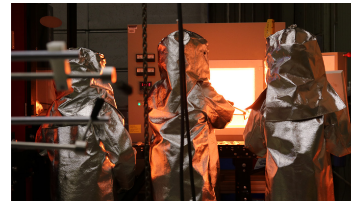
MSU RESEARCHERS HEAT TREAT A STEEL INGOT USING THE REHEAT FURNACE IN THE EDWARDS BUILDING, WHICH IS EQUIPPED FOR HOT- AND COLD-WORKING OF METALS THROUGH ROLLING AND FORGING.
