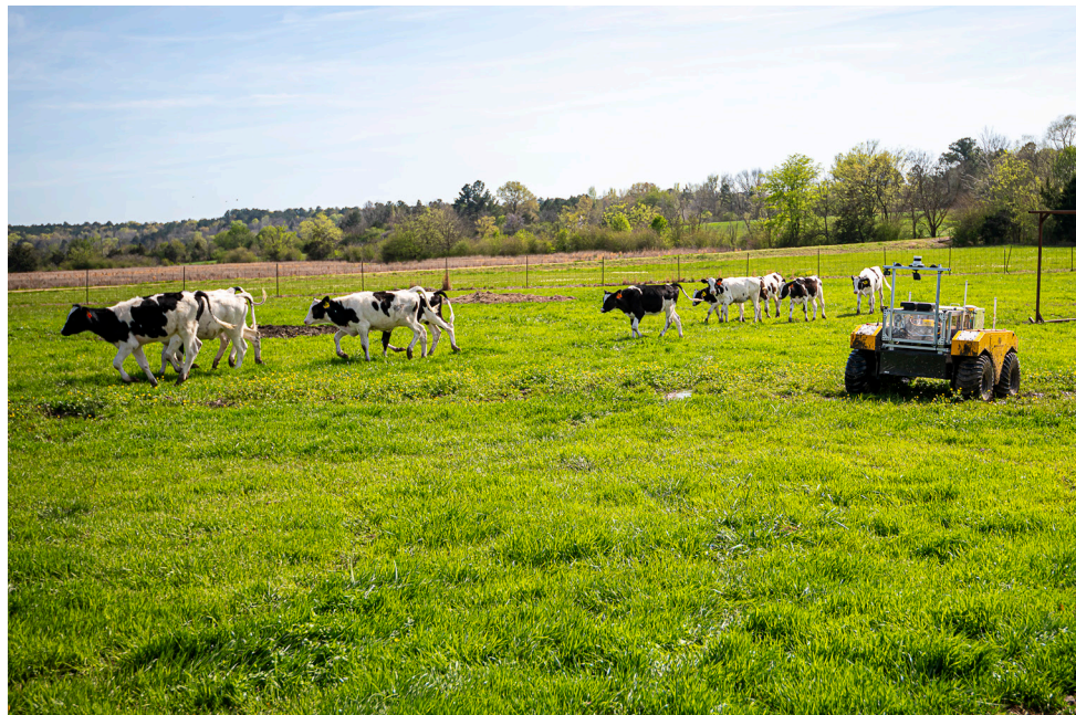
A CLEARPATH ROBOTICS WARTHOG UNCREWED GROUND VEHICLE EQUIPPED WITH CAMERAS AND SENSORS HERDS DAIRY COWS AT MSU'S BEARDEN DAIRY RESEARCH CENTER.
